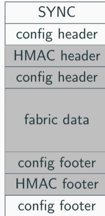
Figure 3: Simplified bitstream format of the Xilinx 7-series - gray parts encrypted [2], [5]
