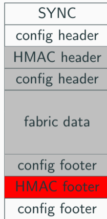
Figure 5: Simplified bitstream format - red part contains authentication-tag [2], [5]
