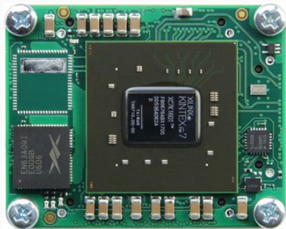
Figure 12: Module with XC7K160T
