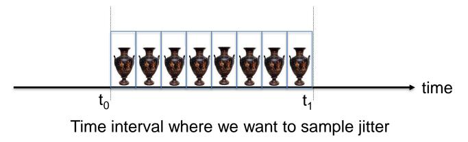
The goal will be to fill this interval with 'transitions' (jitter) of RO outputs, such that any sampling point *t* falls within a 'transition' with high probability.
