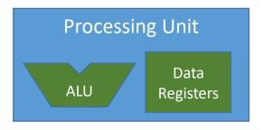
The processing unit constitutes the data path of the CPU
